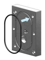
Place a new o-ring on the rear plate.
