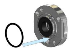
Install a new ring on the sealing unit body.
