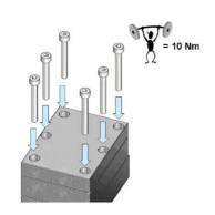
Secure the rear plate with the six screws (tightening torque: 10N.m).
